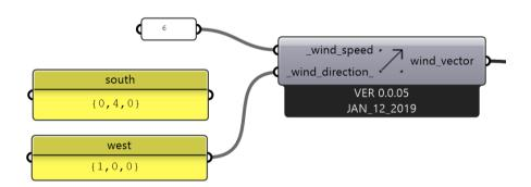
Additionally, wind speed can be changed, and the average wind speed taken from Ladybug's wind rose is used.
