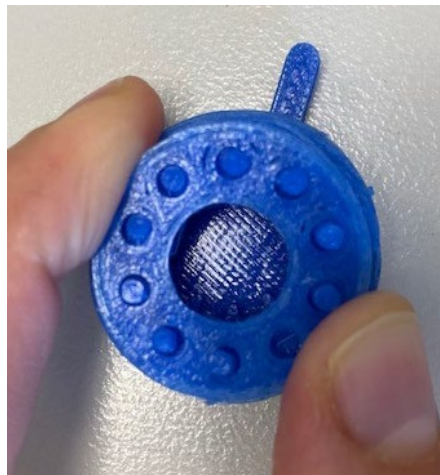
Figure 10. The first 3D printed aperture to test the movement
