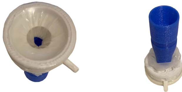
Figure 11. First nozzle design with elastic layer to prevent clay leak into the small parts
