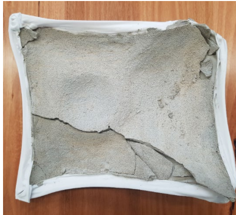
Figure 11. Depicts the stress cracks that lead to the failure of design iteration 4
