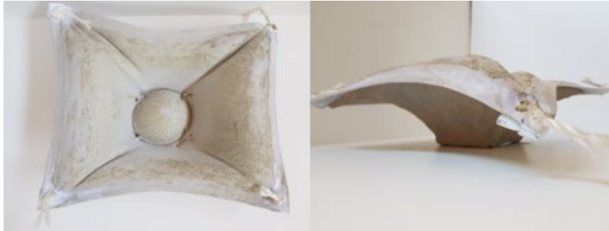
Figure 12. Highlights the 4 small incisions made into the fabric to achieve the overall structure
