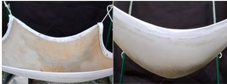
Figure 8. Iteration 3 whilst achieving a very defined form, was unsuccessful due to an inconsistent surface, thinner areas cracked as a result
