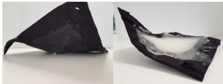
Figure 5. Preliminary wax models that gave valuable insight to how the material properties of the mixture, particularly the viscosity and how this impacted the model
