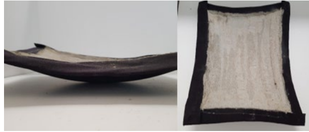
Figure 6. Outcomes of fabricated iteration 2, the first attempt at creating complex geometry using flexible formwork
