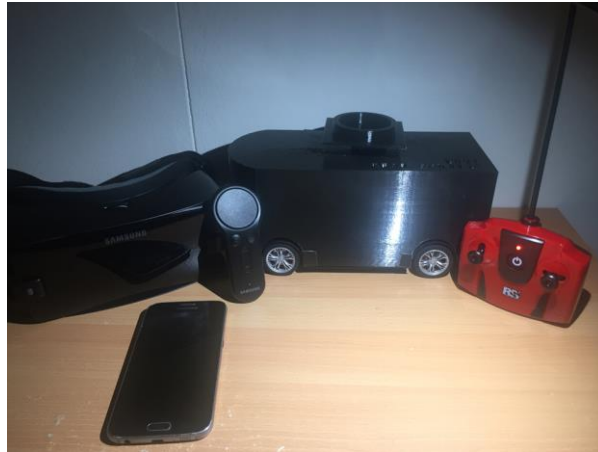
Figure 6. Project setup. Samsung Gear VR with Remote control car with the Arduino components inside, and the rotating platform on top of the car for the 360° camera to sit on top.
