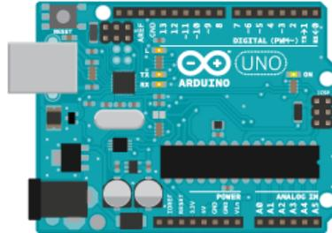
Figure 2. Arduino UNO chipset
