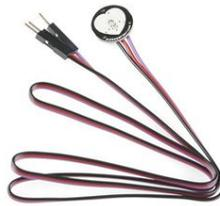
Figure 3. Pulse Sensor Amped module
