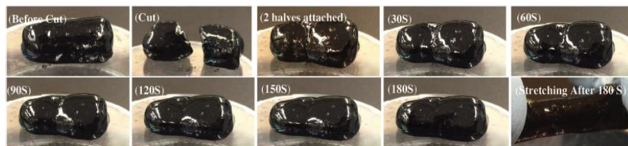
Figure 6. Display of hydrogel-A repairing (image source: Darabi et al., 2017, p.3)
