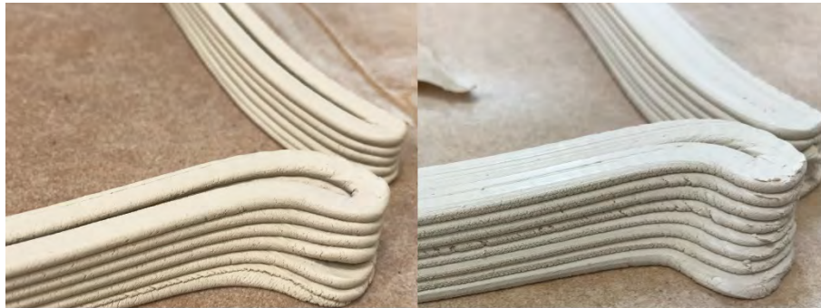
Figure 7. The impact of increasing extrusion width on the separation of the inner and outer walls of the printed model (left) 6mm nozzle and 1.00 x extraction speed; (right) 7.1mm nozzle and 2.00 x extraction speed.
