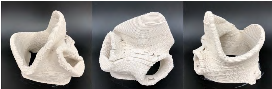
Figure 12. Outcomes of print iteration 8 that involved scoring of the clay. Layer separation particularly evident in the middle image.
