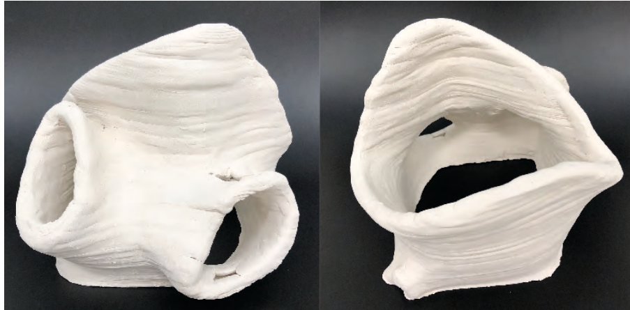
Figure 13. Outcomes of print iteration 9 that involved the pinching and merging of clay layers, the impact of the fabricator evident on the appearance of the clay.
