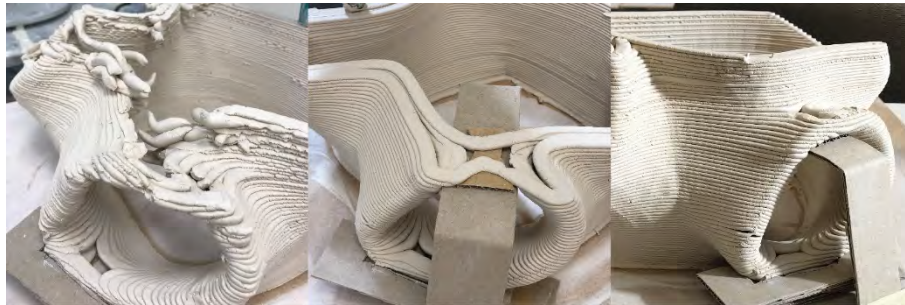
Figure 10. (left) Print outcome with no upper support structure; (middle and right) Photographs showing the use of the upper support structure and the result on print outcomes.
