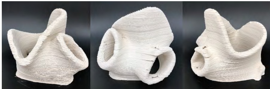
Figure 14. Outcomes of print iteration 10 that involved the application of clay slip between the print layers with a paint brush
