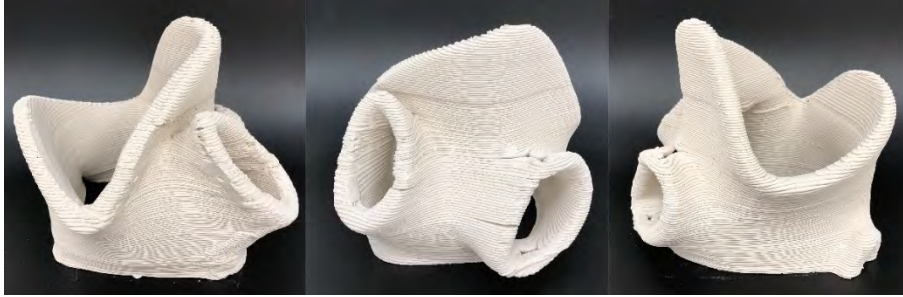
Figure 11. Outcomes of print iteration 7, using supports and intuitive interaction strategies
