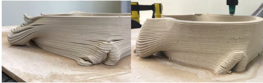
Figure 5. Improvements between two test print iterations realized through the application of the simple human/machine intervention strategies
