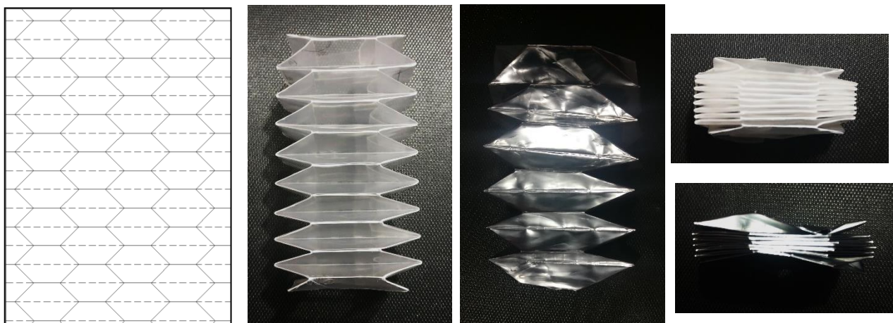
Figure 6 Accordion pattern before folding (left) and after folding using polypropylene (second left) LDPE (middle); after compressed (right- above and below)
