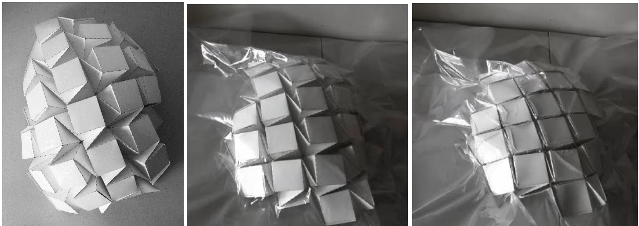
Figure 10 Images showing the deployment and contraction of Square fold pattern
