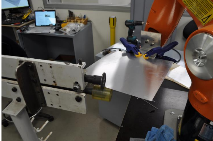
Figure 11 - Image showing the starting position of each robot tooling path for fabrication in process one.
