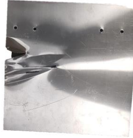
Figure 17 - Image of resulting panel after two iteration test one, success the second iteration, the metal got damaged by the end effector.
