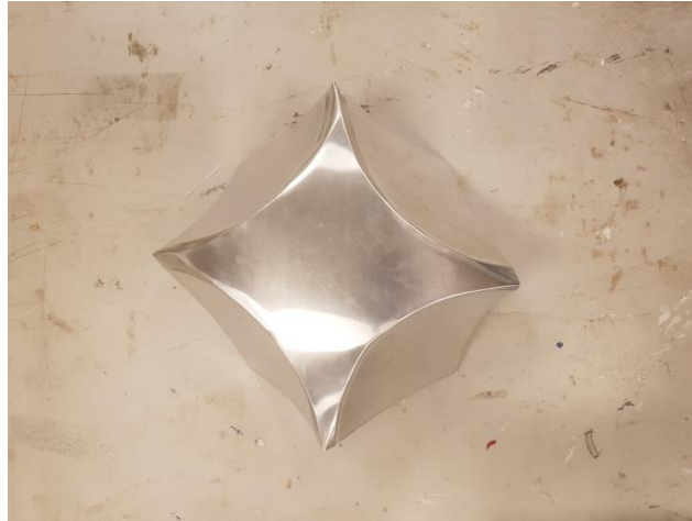
Figure 9 - An image of a bench mark model that aimed to developed four curve creases.
