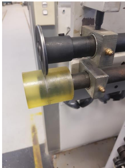
Figure 5 - The forming dies that were used in both process one and two for folding metal up to a 90-degree angle.
