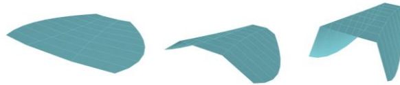
Figure 2 - Three screenshots from the grasshopper that represent the output of the folding process created by kangaroo. This shows the different stages from flat sheet metal to a 3D form.
