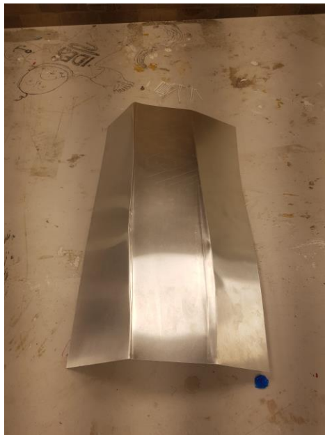
Figure 6 - First benchmark model attempt of two straight line folds.
