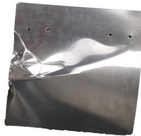
Figure 16 - Image of resulting panel when the end effector in process two got caught on the metal due to bulkiness.
